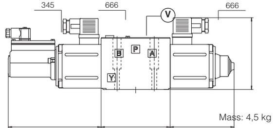
Note: for option /B the solenoid and the position transducer are at side of port A
