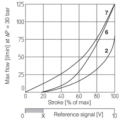
X = Threshold for bias activation depending to the valve type and amplifier type
